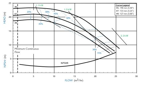
Notes: Performance curves above are based on flooded suction. \*Performance will vary with suction lift conditions. For performance at various suction lifts, see curve book on FTI web site (www.finishthompson.com) or contact factory. Warning! SP Series not recommended for pumping flammables!
